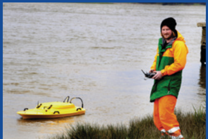
▲ Environmental technical officer Phillip McCartney tests out the remote controlled Q-boat. The high-tech piece of equipment is being used to gather information about the volume and velocity of Southland's rivers to assist with flood forecasting and water quality measurements.
